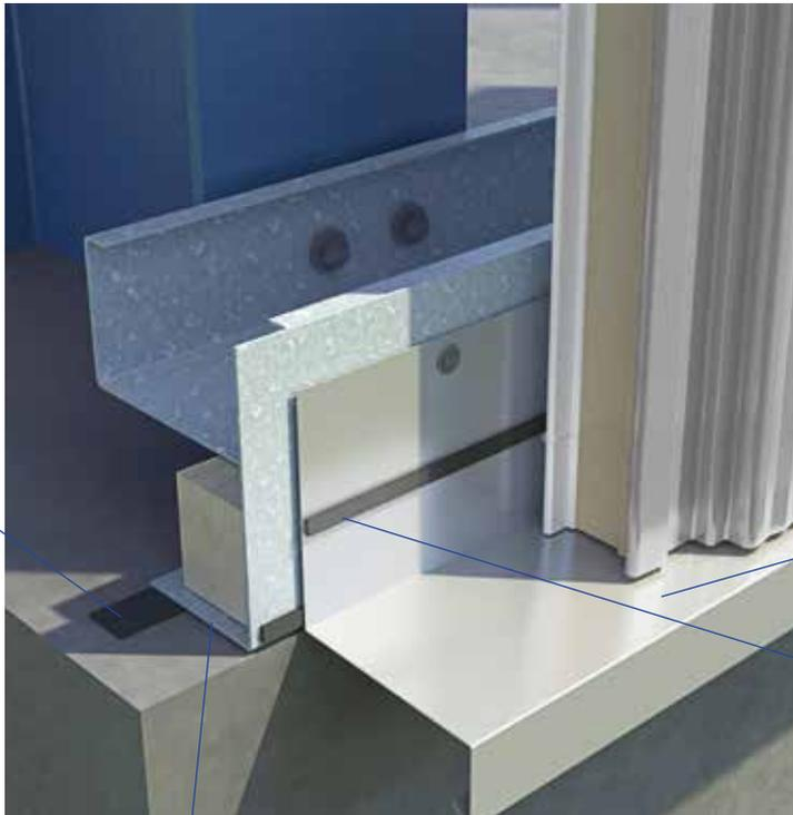
2. Fix the drip support angle to the sheeting rail using low profile fasteners. Ensure the angle compresses the sealant to form a continuous air seal.
