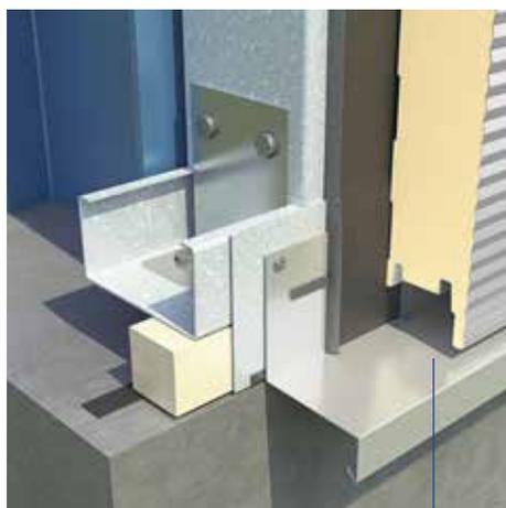
6. Apply a 6mm diameter bead of butyl sealant to the face of the drip support angle. The sealant must meet the bubble gasket.
