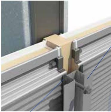
17. Place the top hat flashing into the vertical joint, aligning its base with that of the bottom panel. Fix the top hat flashing to the vertical support at 500mm centres. Ensure the flashing creates an effective weather seal. Do not overdrive the fasteners.
