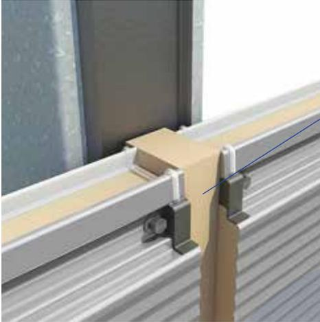
13. Fill the gaps between the panels with PIR insulation board. The depth of the insulation should be cut 30mm less than overall panel thickness to allow clearance for the top hat section.
